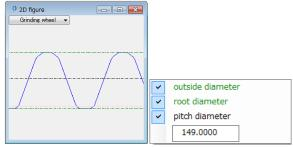
Fig. 13.11 Tooth profile of threaded grinding wheel
