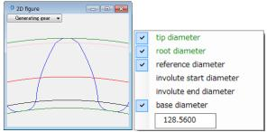
図 13.10 Tooth profile after tooth grinding
