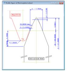
Fig. 13.7 Dimensions of electrodeposition grinding wheel
