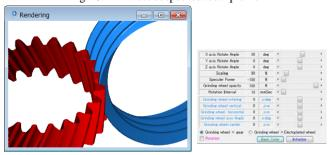
Fig. 13.13 Tooth profile rendering (gear and threaded grinding stone)
